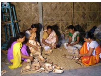
The project envisages use of Arecanut leaves (sheaths), otherwise wasted, for manufacture of arecanut leaf plates and bowls which are eco-friendly, bio-degradable, microwave friendly and can even hold liquids for a few hours.
